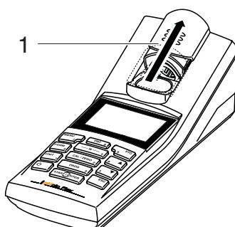
**Inserting a 28 mm cell**
